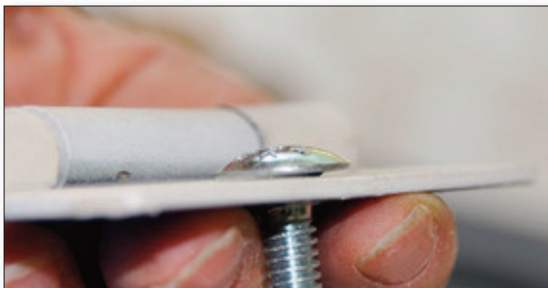
Above: After hole is enlarged, carriage bolt fits flush with hinge surface.
