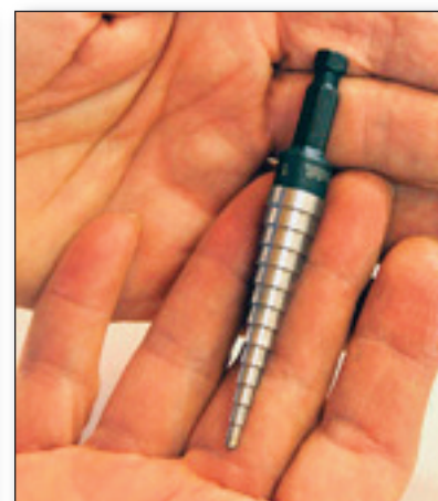
Carriage bolts (left); stepped metal cutting drill bit (above)
